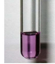
positive biuret test (polypeptide chain chelates with a copper ion)
