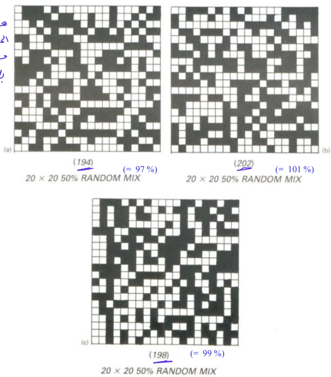
Fig. 32.2 Computer generated mixtures of nominal 50% active ingredient. The numbers in parentheses refer to the number of
