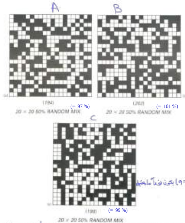
Fig. 10.2 Computer generated mixtures of nominal 50% active ingredients. The number of particles is not necessarily equal to the nominal 50% active ingredient concentration.
