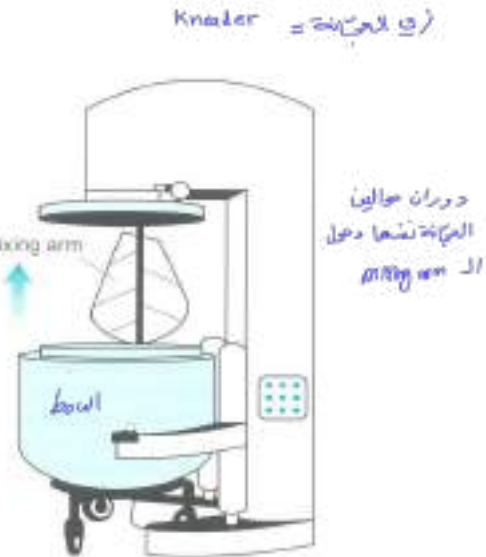
Fig. 12.11 Planetary mixer for powders and semi-solids.
