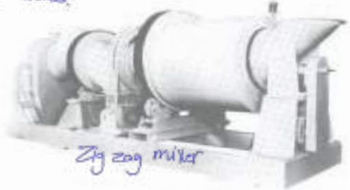
Figure 12 The "Zig Zag" continuous mixer. Courtesy of Farnsworth-Kelly Company, Division of Harsco Corporation, East Stroudsburg, Pennsylvania.
