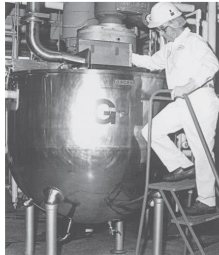
Stainless steel tank, which has counter sweep agitation and a built-in homogenizer.
