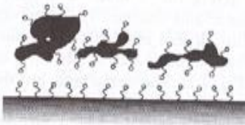
Figure 4.19 Illustrating detergent action. (a) Surface covered with greasy dirt. (b) Detergent is added to the solution. The surfactant molecules reduce adhesion of dirt to the surface when they are deposited with their hydrophobic tails on the solid surface or dirt particle. The dirt particles are thus more easily removed. (c) Detergent molecules solubilize the dirt particles. Dirt particles are held at the surface by the surfactant. [The Estate of I]
