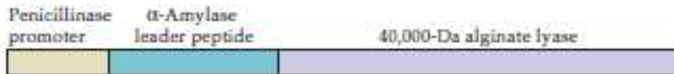
FIGURE 10.16 DNA construct encoding the 40,000-Da alginate lyase. The leader peptide from a B. subtilis \alpha -amylase gene is fused to the N terminus of the alginate lyase coding sequence. The construct is under the transcriptional control of a B. subtilis penicillinase gene expression system.
