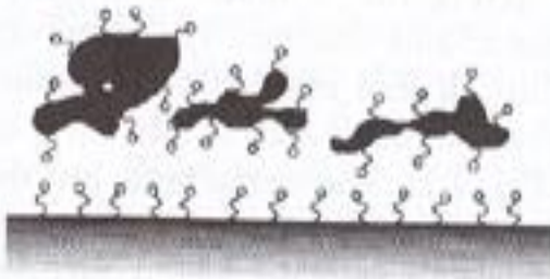
Figure 4.19 Illustrating detergent action. (a) Surface covered with greasy dirt. (b) Detergent is added to the solution. The surfactant molecules reduce adhesion of dirt to the surface when they are deposited with their hydrophobic tails on the solid surface or dirt particle. The dirt particles are thus more readily removed by mechanical action. (c) Dirt particles are held as a suspension by an adsorbed layer of surfactant. [The Estate of Irving Geis]
