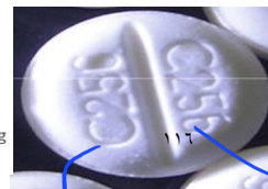
Sticking to punch and picking from tablet
