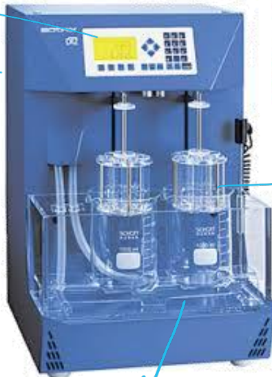
Fig. 31.19 Diagram of a disintegration instrument for the testing of tablet disintegration time.
