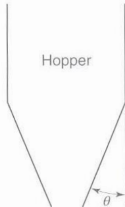
Fig. 13.11 Influence of hopper wall angle and particle-wall friction on powder flow.
