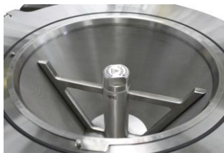
Examples of conical mill impellers
